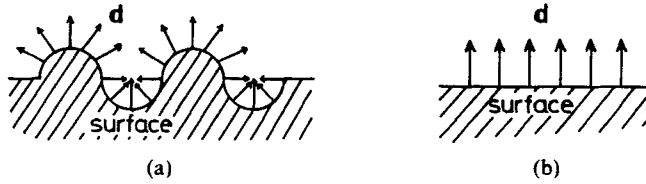
FIGURE 3 (a) The easy axes on the surface having geometrical structure. This figure shows that the easy axes are perpendicular to the local surface. The easy axes are not constant. (b) The easy axes on the flat surface.
